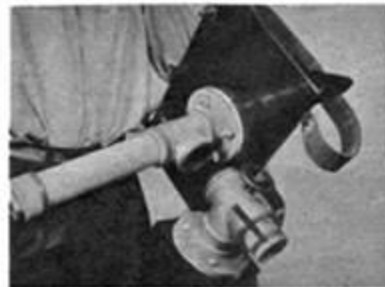
The declination and polar axis. Note the leather straps used to hold tube to saddle.
